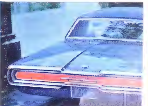
Thunderbird's unique Sequential Turn Signals in full-width taillights signal each turn with a ripple of light.
